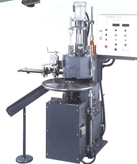
●VG-250S 二頭式縦型バネ両頭研削盤 Vertical Spring End Gringer 2 heads, Single Pass Type
